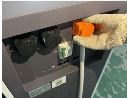
Cover the positive electrode with a protective cover after assembly
