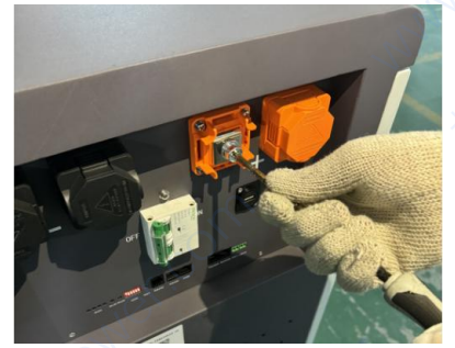
Unscrew the positive screw with a screwdriver
