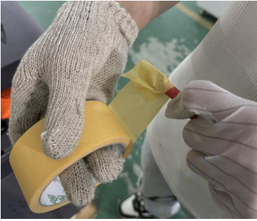
Wear safety gloves and wrap the positive and negative wires with insulating tape Prevent short circuits caused by contact between the positive and negative terminals
