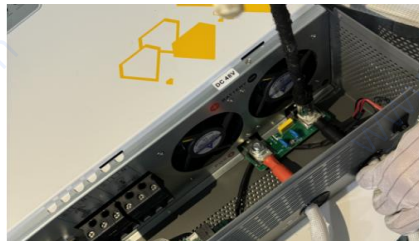
Connect the negative wire of the inverter
