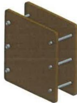
Fig.2 Diagram of the clamp covered with insulation film 2
