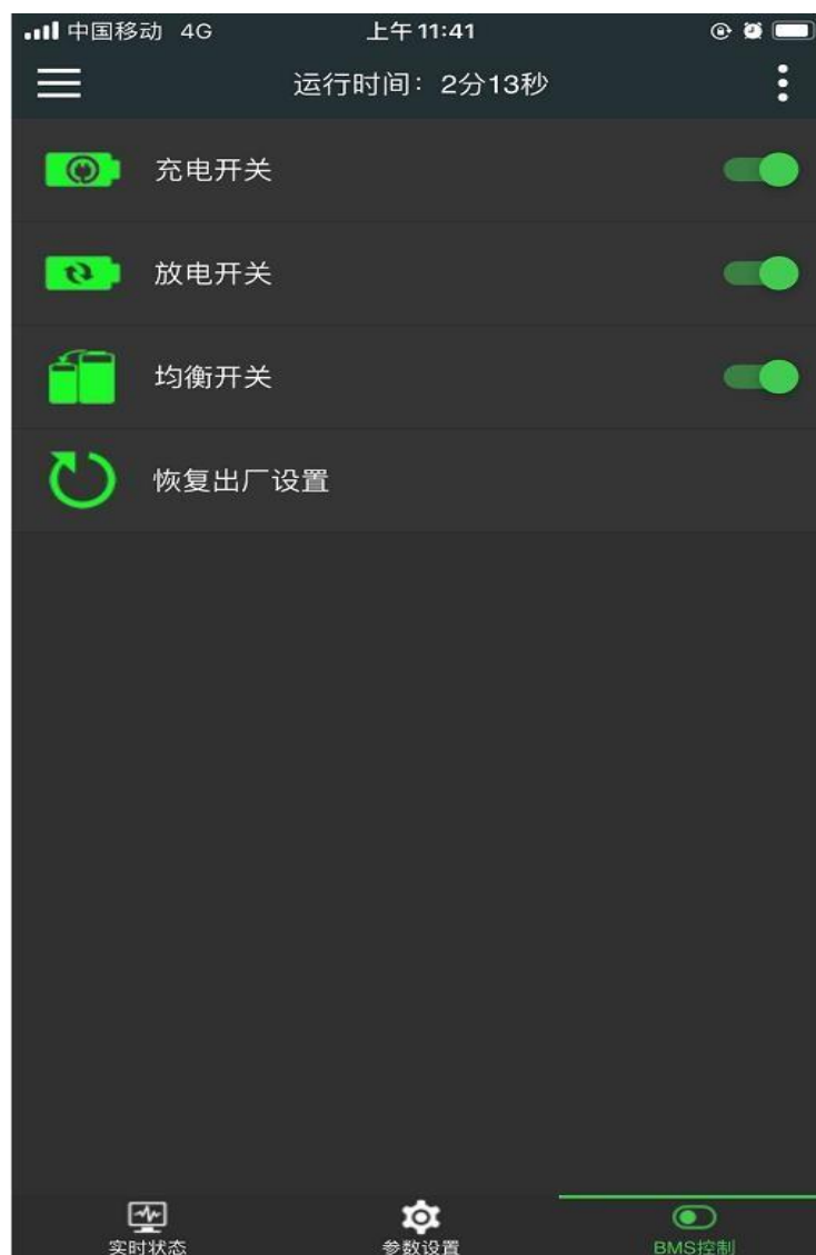
Figure 12 The BMS control page
